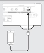
Press DISC/INPUT to select the playback media mode to "iPod/USB".
